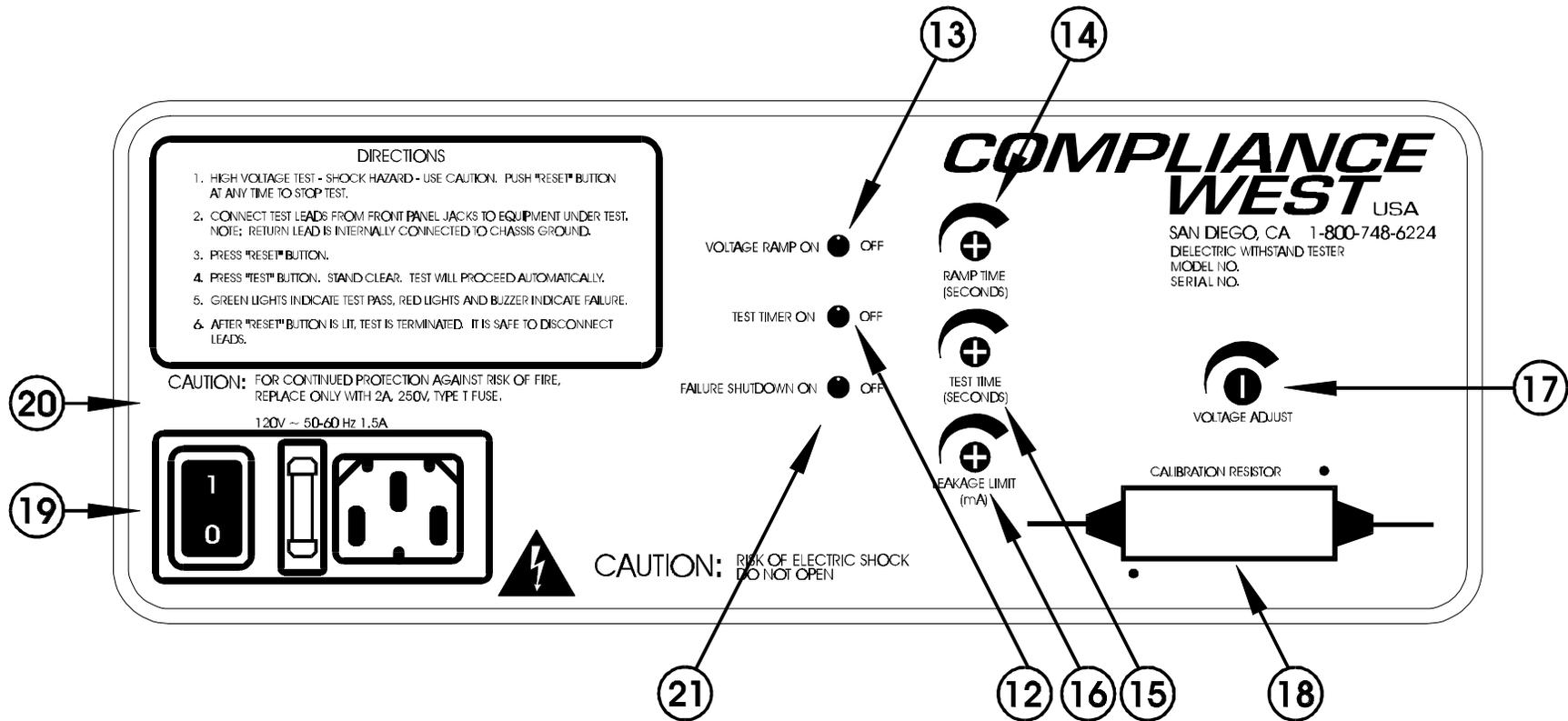
Figure 3-2. Controls, Indicators, Connectors - Model HT-5000 Rear Panel
