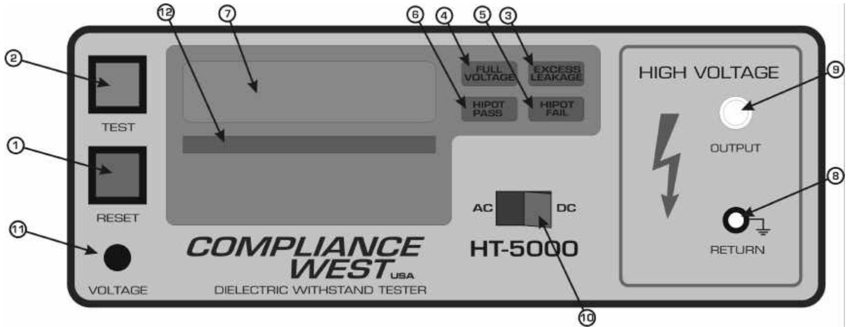
Figure 3-1. Controls, Indicators, Connectors - Model HT-5000 Front Panel
